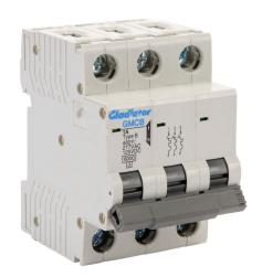
Gladiator miniature supplementary protector, 1A, 480Y / 277 VAC / 125 VDC, 3-pole, B curve, thermal magnetic, 6kA @ 480Y/277 VAC interrupting rating, 35mm DIN rail mount.
