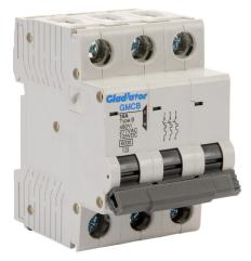
Gladiator miniature supplementary protector, 16A, 480Y / 277 VAC / 125 VDC, 3-pole, B curve, thermal magnetic, 6kA @ 480Y/277 VAC interrupting rating, 35mm DIN rail mount.
