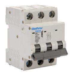
Gladiator miniature supplementary protector, 15A, 480Y / 277 VAC / 125 VDC, 3-pole, B curve, thermal magnetic, 6kA @ 480Y/277 VAC interrupting rating, 35mm DIN rail mount.
