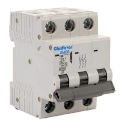
Gladiator miniature supplementary protector, 10A, 480Y / 277 VAC / 125 VDC, 3-pole, B curve, thermal magnetic, 6kA @ 480Y/277 VAC interrupting rating, 35mm DIN rail mount.
