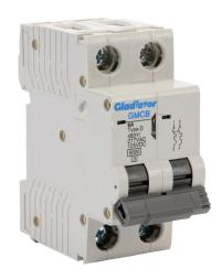
Gladiator miniature supplementary protector, 8A, 480Y / 277 VAC / 125 VDC, 2-pole, D curve, thermal magnetic, 6kA @ 480Y/277 VAC interrupting rating, 35mm DIN rail mount.
