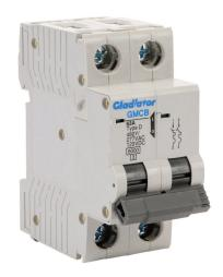
Gladiator miniature supplementary protector, 63A, 480Y / 277 VAC / 125 VDC, 2-pole, D curve, thermal magnetic, 6kA @ 480Y/277 VAC interrupting rating, 35mm DIN rail mount.
