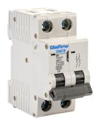
Gladiator miniature supplementary protector, 5A, 480Y / 277 VAC / 125 VDC, 2-pole, D curve, thermal magnetic, 6kA @ 480Y/277 VAC interrupting rating, 35mm DIN rail mount.
