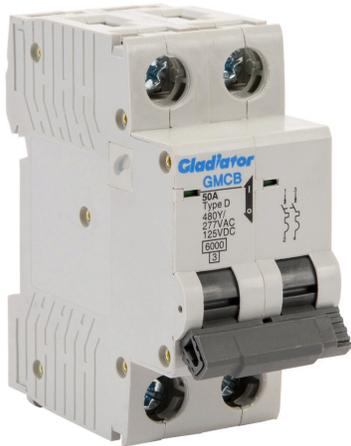
Gladiator miniature supplementary protector, 50A, 480Y / 277 VAC / 125 VDC, 2-pole, D curve, thermal magnetic, 6kA @ 480Y/277 VAC interrupting rating, 35mm DIN rail mount.
