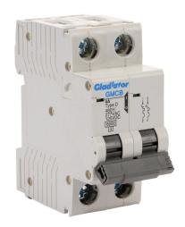
Gladiator miniature supplementary protector, 4A, 480Y / 277 VAC / 125 VDC, 2-pole, D curve, thermal magnetic, 6kA @ 480Y/277 VAC interrupting rating, 35mm DIN rail mount.
