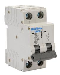
Gladiator miniature supplementary protector, 40A, 480Y / 277 VAC / 125 VDC, 2-pole, D curve, thermal magnetic, 6kA @ 480Y/277 VAC interrupting rating, 35mm DIN rail mount.
