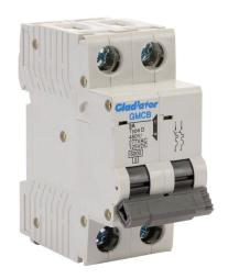
Gladiator miniature supplementary protector, 3A, 480Y / 277 VAC / 125 VDC, 2-pole, D curve, thermal magnetic, 6kA @ 480Y/277 VAC interrupting rating, 35mm DIN rail mount.
