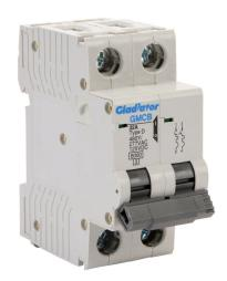
Gladiator miniature supplementary protector, 32A, 480Y / 277 VAC / 125 VDC, 2-pole, D curve, thermal magnetic, 6kA @ 480Y/277 VAC interrupting rating, 35mm DIN rail mount.
