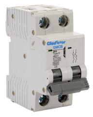
Gladiator miniature supplementary protector, 30A, 480Y / 277 VAC / 125 VDC, 2-pole, D curve, thermal magnetic, 6kA @ 480Y/277 VAC interrupting rating, 35mm DIN rail mount.
