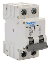
Gladiator miniature supplementary protector, 25A, 480Y / 277 VAC / 125 VDC, 2-pole, D curve, thermal magnetic, 6kA @ 480Y/277 VAC interrupting rating, 35mm DIN rail mount.
