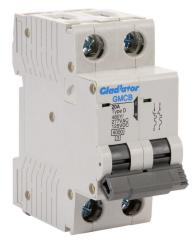
Gladiator miniature supplementary protector, 20A, 480Y / 277 VAC / 125 VDC, 2-pole, D curve, thermal magnetic, 6kA @ 480Y/277 VAC interrupting rating, 35mm DIN rail mount.
