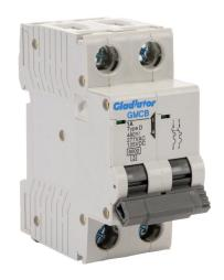
Gladiator miniature supplementary protector, 1A, 480Y / 277 VAC / 125 VDC, 2-pole, D curve, thermal magnetic, 6kA @ 480Y/277 VAC interrupting rating, 35mm DIN rail mount.
