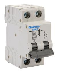
Gladiator miniature supplementary protector, 16A, 480Y / 277 VAC / 125 VDC, 2-pole, D curve, thermal magnetic, 6kA @ 480Y/277 VAC interrupting rating, 35mm DIN rail mount.
