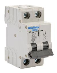
Gladiator miniature supplementary protector, 15A, 480Y / 277 VAC / 125 VDC, 2-pole, D curve, thermal magnetic, 6kA @ 480Y/277 VAC interrupting rating, 35mm DIN rail mount.
