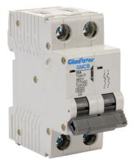
Gladiator miniature supplementary protector, 10A, 480Y / 277 VAC / 125 VDC, 2-pole, D curve, thermal magnetic, 6kA @ 480Y/277 VAC interrupting rating, 35mm DIN rail mount.
