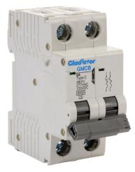
Gladiator miniature supplementary protector, 8A, 480Y / 277 VAC / 125 VDC, 2-pole, C curve, thermal magnetic, 6kA @ 480Y/277 VAC interrupting rating, 35mm DIN rail mount.
