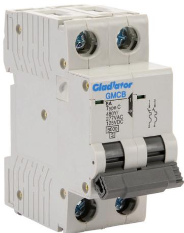
Gladiator miniature supplementary protector, 6A, 480Y / 277 VAC / 125 VDC, 2-pole, C curve, thermal magnetic, 6kA @ 480Y/277 VAC interrupting rating, 35mm DIN rail mount.
