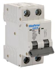
Gladiator miniature supplementary protector, 63A, 480Y / 277 VAC / 125 VDC, 2-pole, C curve, thermal magnetic, 6kA @ 480Y/277 VAC interrupting rating, 35mm DIN rail mount.
