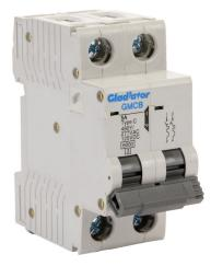
Gladiator miniature supplementary protector, 5A, 480Y / 277 VAC / 125 VDC, 2-pole, C curve, thermal magnetic, 6kA @ 480Y/277 VAC interrupting rating, 35mm DIN rail mount.
