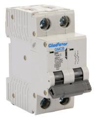
Gladiator miniature supplementary protector, 50A, 480Y / 277 VAC / 125 VDC, 2-pole, C curve, thermal magnetic, 6kA @ 480Y/277 VAC interrupting rating, 35mm DIN rail mount.
