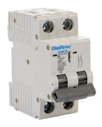
Gladiator miniature supplementary protector, 4A, 480Y / 277 VAC / 125 VDC, 2-pole, C curve, thermal magnetic, 6kA @ 480Y/277 VAC interrupting rating, 35mm DIN rail mount.
