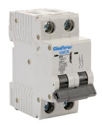
Gladiator miniature supplementary protector, 40A, 480Y / 277 VAC / 125 VDC, 2-pole, C curve, thermal magnetic, 6kA @ 480Y/277 VAC interrupting rating, 35mm DIN rail mount.
