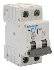
Gladiator miniature supplementary protector, 3A, 480Y / 277 VAC / 125 VDC, 2-pole, C curve, thermal magnetic, 6kA @ 480Y/277 VAC interrupting rating, 35mm DIN rail mount.
