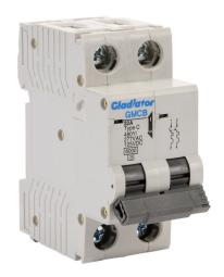
Gladiator miniature supplementary protector, 32A, 480Y / 277 VAC / 125 VDC, 2-pole, C curve, thermal magnetic, 6kA @ 480Y/277 VAC interrupting rating, 35mm DIN rail mount.
