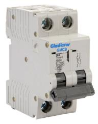
Gladiator miniature supplementary protector, 30A, 480Y / 277 VAC / 125 VDC, 2-pole, C curve, thermal magnetic, 6kA @ 480Y/277 VAC interrupting rating, 35mm DIN rail mount.
