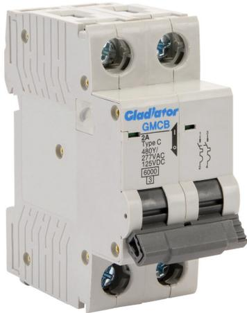
Gladiator miniature supplementary protector, 2A, 480Y / 277 VAC / 125 VDC, 2-pole, C curve, thermal magnetic, 6kA @ 480Y/277 VAC interrupting rating, 35mm DIN rail mount.
