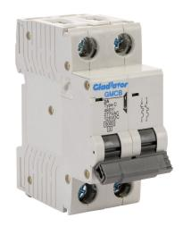
Gladiator miniature supplementary protector, 2A, 480Y / 277 VAC / 125 VDC, 2-pole, C curve, thermal magnetic, 6kA @ 480Y/277 VAC interrupting rating, 35mm DIN rail mount.
