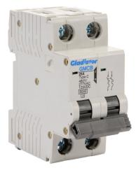
Gladiator miniature supplementary protector, 25A, 480Y / 277 VAC / 125 VDC, 2-pole, C curve, thermal magnetic, 6kA @ 480Y/277 VAC interrupting rating, 35mm DIN rail mount.
