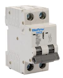
Gladiator miniature supplementary protector, 20A, 480Y / 277 VAC / 125 VDC, 2-pole, C curve, thermal magnetic, 6kA @ 480Y/277 VAC interrupting rating, 35mm DIN rail mount.
