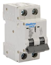
Gladiator miniature supplementary protector, 1A, 480Y / 277 VAC / 125 VDC, 2-pole, C curve, thermal magnetic, 6kA @ 480Y/277 VAC interrupting rating, 35mm DIN rail mount.
