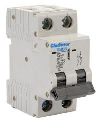
Gladiator miniature supplementary protector, 16A, 480Y / 277 VAC / 125 VDC, 2-pole, C curve, thermal magnetic, 6kA @ 480Y/277 VAC interrupting rating, 35mm DIN rail mount.
