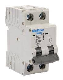
Gladiator miniature supplementary protector, 15A, 480Y / 277 VAC / 125 VDC, 2-pole, C curve, thermal magnetic, 6kA @ 480Y/277 VAC interrupting rating, 35mm DIN rail mount.
