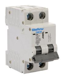
Gladiator miniature supplementary protector, 10A, 480Y / 277 VAC / 125 VDC, 2-pole, C curve, thermal magnetic, 6kA @ 480Y/277 VAC interrupting rating, 35mm DIN rail mount.
