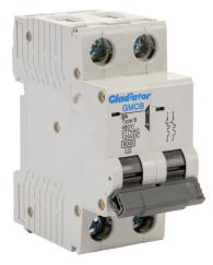
Gladiator miniature supplementary protector, 8A, 480Y / 277 VAC / 125 VDC, 2-pole, B curve, thermal magnetic, 6kA @ 480Y/277 VAC interrupting rating, 35mm DIN rail mount.
