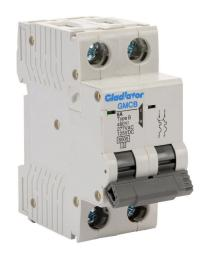
Gladiator miniature supplementary protector, 6A, 480Y / 277 VAC / 125 VDC, 2-pole, B curve, thermal magnetic, 6kA @ 480Y/277 VAC interrupting rating, 35mm DIN rail mount.
