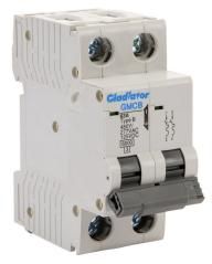
Gladiator miniature supplementary protector, 63A, 480Y / 277 VAC / 125 VDC, 2-pole, B curve, thermal magnetic, 6kA @ 480Y/277 VAC interrupting rating, 35mm DIN rail mount.
