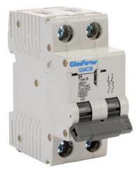
Gladiator miniature supplementary protector, 5A, 480Y / 277 VAC / 125 VDC, 2-pole, B curve, thermal magnetic, 6kA @ 480Y/277 VAC interrupting rating, 35mm DIN rail mount.
