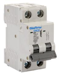
Gladiator miniature supplementary protector, 50A, 480Y / 277 VAC / 125 VDC, 2-pole, B curve, thermal magnetic, 6kA @ 480Y/277 VAC interrupting rating, 35mm DIN rail mount.
