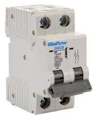
Gladiator miniature supplementary protector, 4A, 480Y / 277 VAC / 125 VDC, 2-pole, B curve, thermal magnetic, 6kA @ 480Y/277 VAC interrupting rating, 35mm DIN rail mount.
