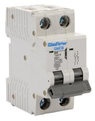
Gladiator miniature supplementary protector, 40A, 480Y / 277 VAC / 125 VDC, 2-pole, B curve, thermal magnetic, 6kA @ 480Y/277 VAC interrupting rating, 35mm DIN rail mount.
