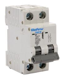
Gladiator miniature supplementary protector, 3A, 480Y / 277 VAC / 125 VDC, 2-pole, B curve, thermal magnetic, 6kA @ 480Y/277 VAC interrupting rating, 35mm DIN rail mount.
