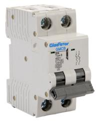
Gladiator miniature supplementary protector, 32A, 480Y / 277 VAC / 125 VDC, 2-pole, B curve, thermal magnetic, 6kA @ 480Y/277 VAC interrupting rating, 35mm DIN rail mount.
