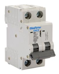
Gladiator miniature supplementary protector, 30A, 480Y / 277 VAC / 125 VDC, 2-pole, B curve, thermal magnetic, 6kA @ 480Y/277 VAC interrupting rating, 35mm DIN rail mount.
