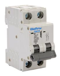
Gladiator miniature supplementary protector, 2A, 480Y / 277 VAC / 125 VDC, 2-pole, B curve, thermal magnetic, 6kA @ 480Y/277 VAC interrupting rating, 35mm DIN rail mount.
