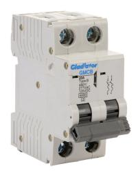
Gladiator miniature supplementary protector, 20A, 480Y / 277 VAC / 125 VDC, 2-pole, B curve, thermal magnetic, 6kA @ 480Y/277 VAC interrupting rating, 35mm DIN rail mount.
