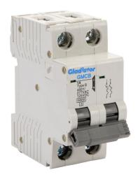
Gladiator miniature supplementary protector, 1A, 480Y / 277 VAC / 125 VDC, 2-pole, B curve, thermal magnetic, 6kA @ 480Y/277 VAC interrupting rating, 35mm DIN rail mount.
