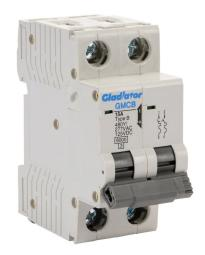
Gladiator miniature supplementary protector, 15A, 480Y / 277 VAC / 125 VDC, 2-pole, B curve, thermal magnetic, 6kA @ 480Y/277 VAC interrupting rating, 35mm DIN rail mount.
